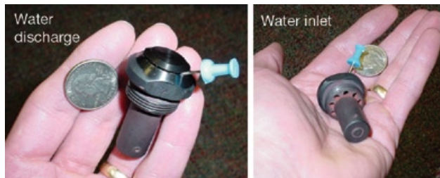
2. Spray-nozzle openings are extremely small. Tack holds nozzles at near its full-open position
