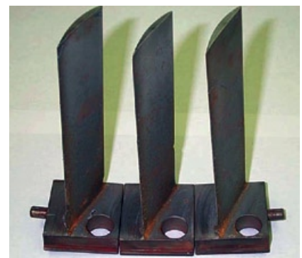
3. Pinned blades still "rock solid" after 700 starts and 8000 hours in service, despite heavy foreign object damage
