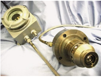
5. Optically instrumented fuel nozzle (foreground) is linked to signal processor at left by fiber optic cable
