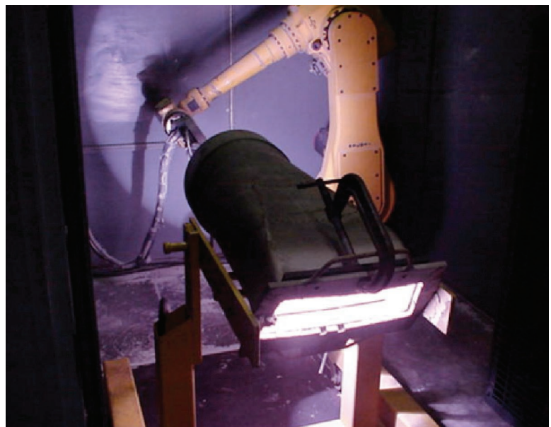
6. Robotic coating application helps improve component design life
